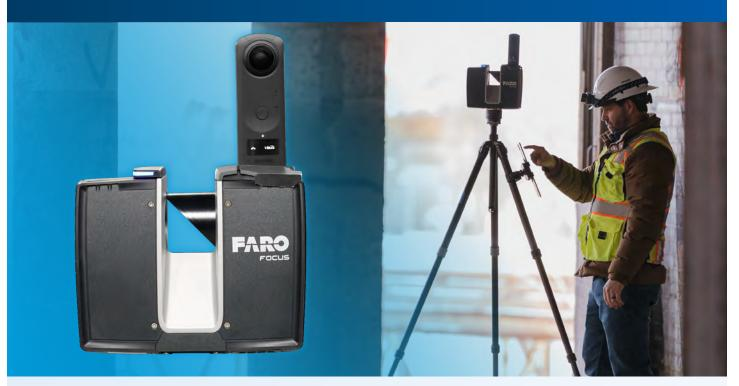
The FARO Focus Premium creates accurate, photorealistic 3D representations of any environment or object in just a few minutes – even in the most extreme outdoors conditions. For best on-site data capture, Focus Premium connects with the FARO Stream app, bridging FARO hardware to the FARO Sphere cloud environment. Pre-registration scans are fed directly into the cloud, so jobs can be done more efficiently.
